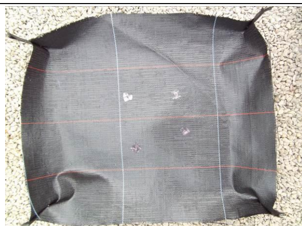
Figure 2. Squares of woven ground cover inoculated with either Pythium or Fusarium mycelium, prior to treatment
